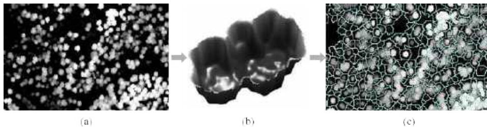
(a) CHM; (b) Watershed Segmentation Algorithm; (c) CHM Segmentation Result
